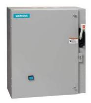
2-speed 3-phase motor starter, Size 0, Two separate windings, Constant or variable torque, Solid-state overload relays, Low spd OLR range 0.25-1A, High Spd OLR range 0.75-3.4A, 24VAC 50-60Hz coil, Combination type, 30A disconnect switch, Enclosure NEMA type 1, Indoor general purpose use
