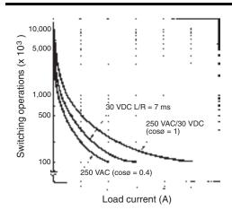
**Reference:** A maximum current of 0.15 A can be switched at 125 VDC ( $\cos\phi = 1$ ) and a maximum current of 0.1 A can be switched at 125 VDC and L/R = 7ms. In both cases, a life of 100,000 operations can be expected. The minimum applicable load is 10 mA at 5 VDC (failure level: P).
