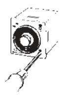
For OFF-time, the desired time unit (sec, 10 s, min, and hrs, or 10 s, 10 min, hrs, and 10 h) is indicated in the OFF-time unit display window at the upper right corner of the front panel and can be changed by turning the OFF-time unit selector located below the OFF-time unit display window.
