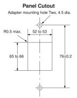
**Note:** The mounting panel thickness should be 1 to 3.2 mm.
