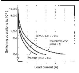
**Reference:** A maximum current of 0.15 A can be switched at 125 VDC ( $\cos\phi = 1$ ) and a maximum current of 0.1 A can be switched at 125 VDC and L/R = 7ms. In both cases, a life of 100,000 operations can be expected. The minimum applicable load is 100 mA at 5 VDC (failure level: P).
