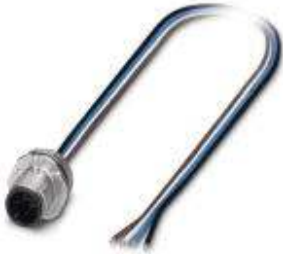
Sensor/Actuator flush-type plug, 4-pos., M12-SPEEDCON, A-coded, front/screw mounting with M16 thread, with 0.5 m TPE litz wire, 4 x 0.34 mm 2
