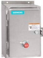
Non-reversing motor starter Size 0 Three phase full voltage Solid-state overload relay OLRelay amp range 0.25-1A 220-240/440-480VAC 60HZ coil Combination type Water/dust tight non-corrosive
