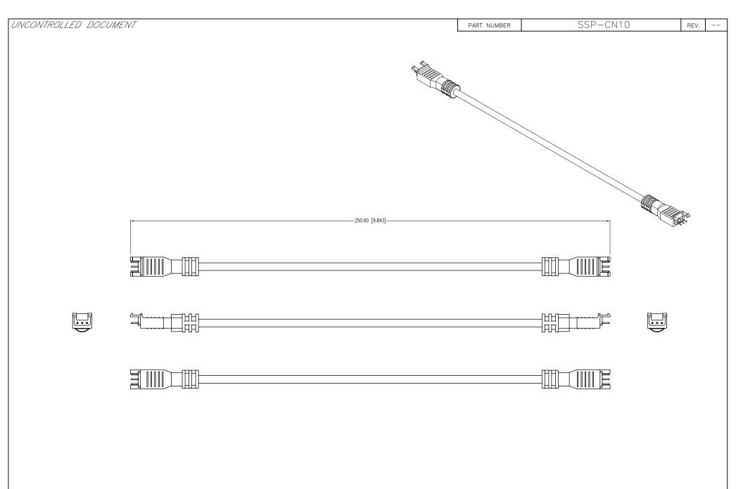
\*UNLESS OTHERWISE SPECIFIED TOLERANCES PER DECIMAL PRECISION ARE: X=±1 (±0.039), X.X=±0.5 (±0.020), X.XX=±0.25 (±0.010), X.XXX=±0.127 (±0.005). LEAD SIZE=±0.05 (±0.002), LEAD LENGTH=±0.75 (±0.030). MIN=  $^{+0.00}_{-0.00}$  MAX.=  $^{+0.00}_{-0.00}$  MAX.=  $^{+0.00}_{-0.00}$  PRECISION UNCONTROUED DOCUMENT
