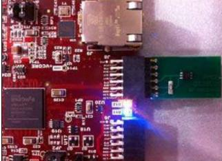
Note: The DS28E01PMOD is designed to plug in componentside up of the upper row pins on the J8 connector, when using the Xilinx Spartan-6 LX16 Evaluation Kit.
