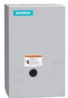
Non-reversing contactor, Size 2 1/2, Single phase full voltage, Contactor amp rating 60A, 3 wire (NO aux included), 220-240/440-480VAC 60Hz coil, Noncombination type, Enclosure NEMA type 1, Indoor general purpose use, Standard width enclosure
