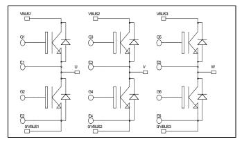
$V_{CES} = 1200V$  $I_{C} = 75A$  @  $T_{C} = 80^{\circ}C$
