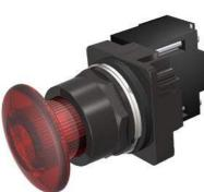
30mm BlackMax, Epoxy Coated Corrosion Resistant Complete Metal Unit Illuminated Push-Pull Operator Transformer type, 480V AC LED Lamp Mushroom Head Cap Small 1 3/4" (44.5 mm) Plastic, Red 3 Position Momentary UL Listed, CSA Certified NEMA 1,3,3R,4,4X,12,13 & Automotive Standards
