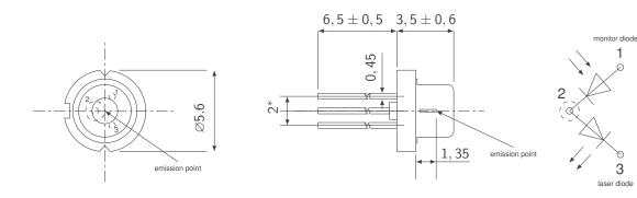
all dimensions in mm. Tolerance  $\pm 0,\,2$  except given ones \* at the bottom of the LED
