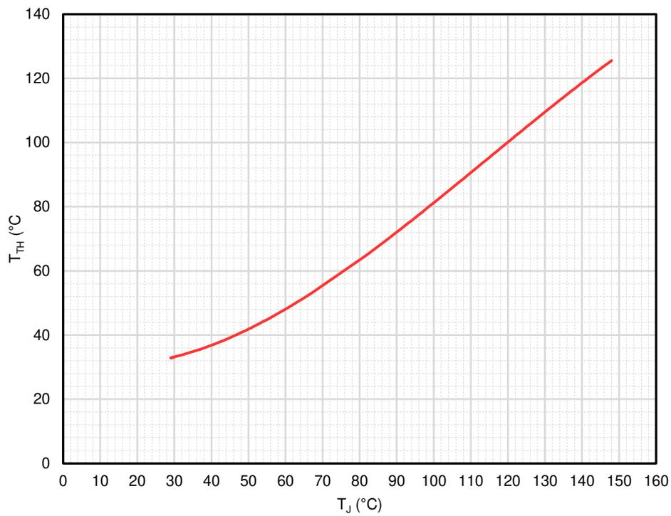
**Figure 9:** T<sub>TH</sub> vs T<sub>J</sub> for a module without a heat sink. V<sub>CC</sub>=15.4V, R=7.50kΩ
