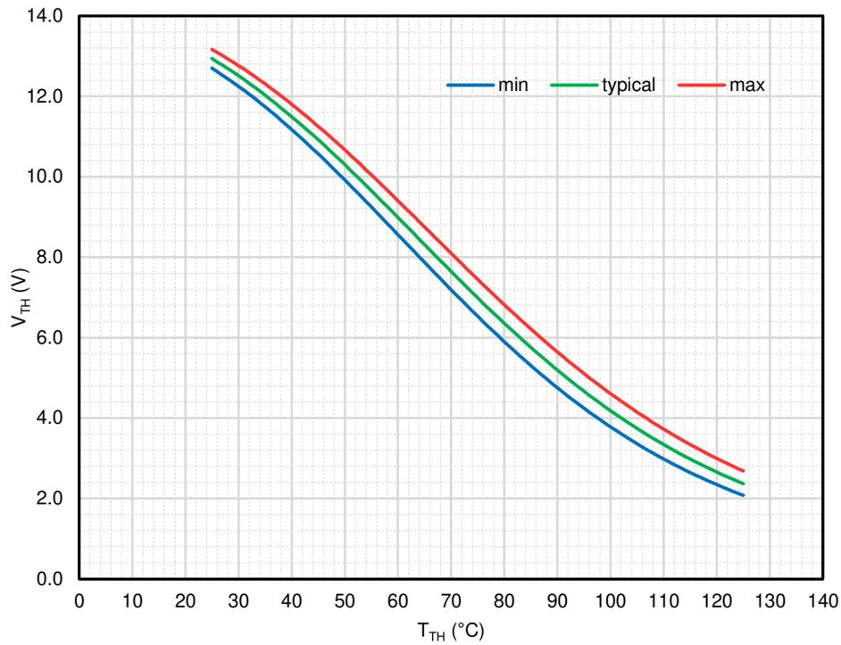
**Figure 8:** V<sub>TH</sub> vs T<sub>TH</sub> with V<sub>TH</sub> pin pulled up to V<sub>CC</sub> with a 7.50kΩ (1%, 100ppm) resistor. A 15V, 1% variation in V<sub>CC</sub> is assumed.
