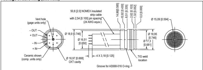
Note: Non-concentricity effects at the diaphragm weld area may cause runout of up to ±0.006 in between the upper and lower portions of the sensor body. (It is recommended to use a counter bore to mate with this device to allow for this non-concentricity).
