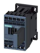
power contactor, AC-3e/AC-3, 7 A, 3 kW / 400 V, 3-pole, 110 V AC, 50 Hz / 120 V, 60 Hz, with plugged-on RC element, auxiliary contacts: 1 NO, spring-loaded terminal, size: S00
