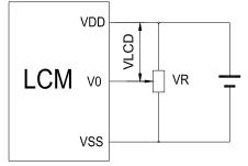
$V_{DD-}V_0$ : LCD Driving voltage VR: 10k~20k
