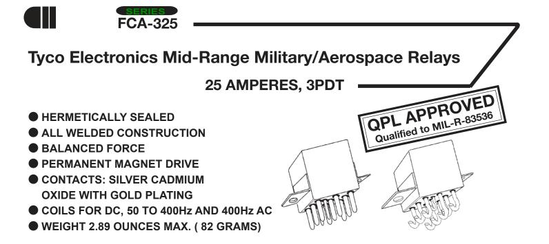
The Series FCA-325 relay is a polarized single-side stable design, where the flux from a permanent magnet provides the armature holding force in the deactivated state, and its flux path is switched and combined with the coil flux in the operated state. This results in appreciably increased contact pressure in both states over that of a spring return nonpolar design. We also manufacture other versions of this relay:
