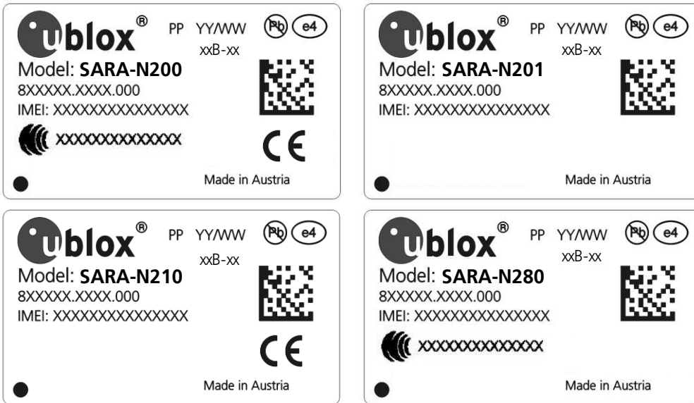
Figure 7 Location of product type number on SARA-N2 series module label
