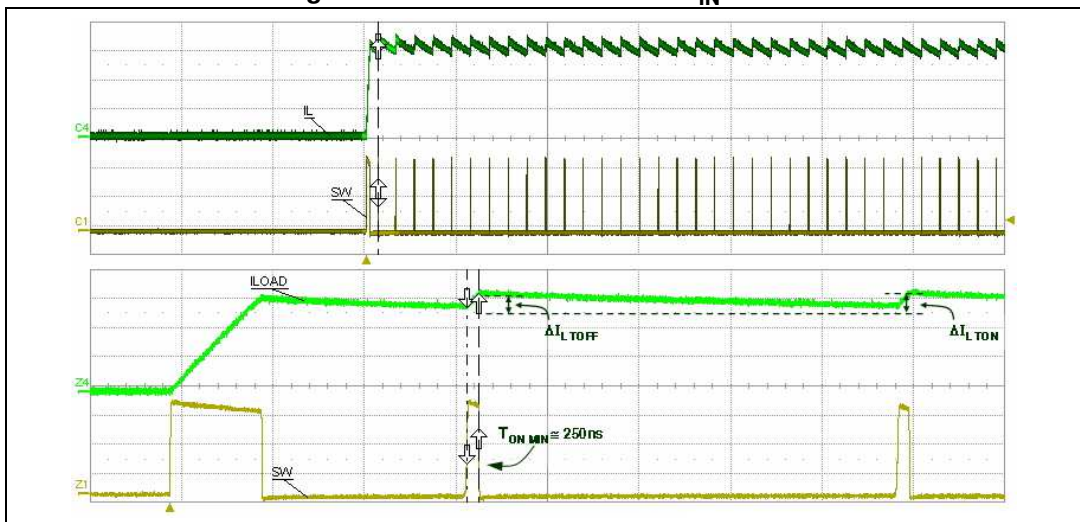
Figure 21. Short-circuit current V_{IN} = 36\text{ V}
