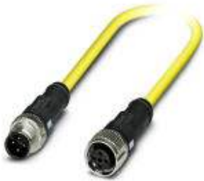
Sensor/Actuator cable, 4-position, TPE, yellow RAL 1021, Plug straight M12 SPEEDCON, A-coded, on Socket straight M12 SPEEDCON, A-coded, Cable length: 5 m
