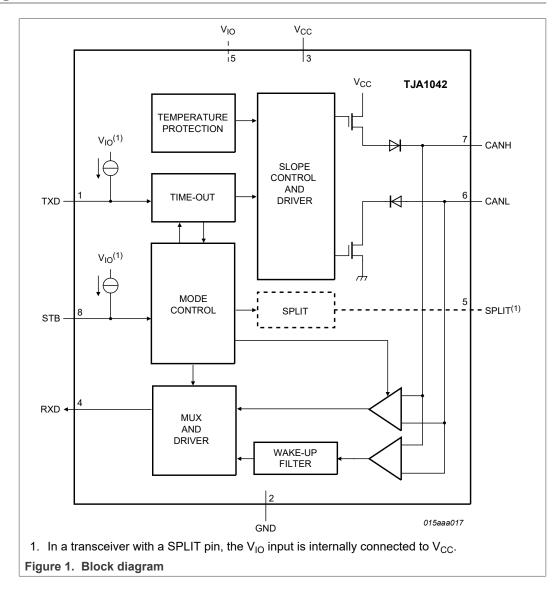
High-speed CAN transceiver with Standby mode
