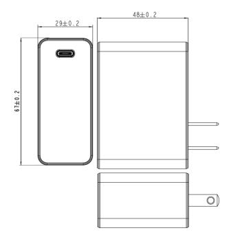
AQ36E-5CA-H Dimension Diagram Unit: mm
