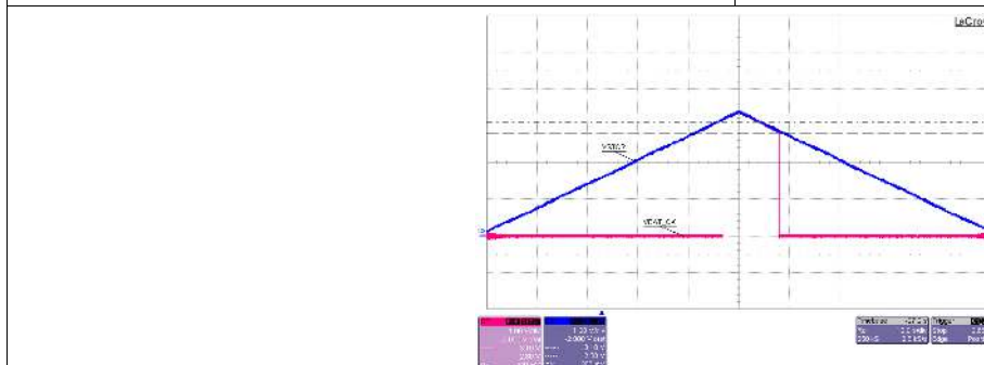
VIN\_DC floating No storage element on V_{BAT} or V_{BAT\_PRI} V_{STOR} artificially ramped from 0\text{ V} to 3.3\text{ V} to 0\text{ V} using a function generator
