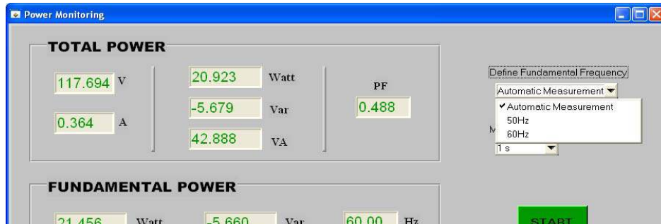
Figure 14. Power Monitoring Window, Define Fundamental Frequency Menu
