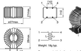
Recommended hole diameter: ød+0.5 Dimensions in mm
