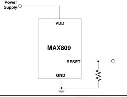
Microprocessor voltage detection reset chip
