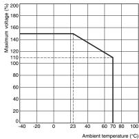
Note. The maximum voltage is the maximum voltage that can be applied to the relay cooil.
