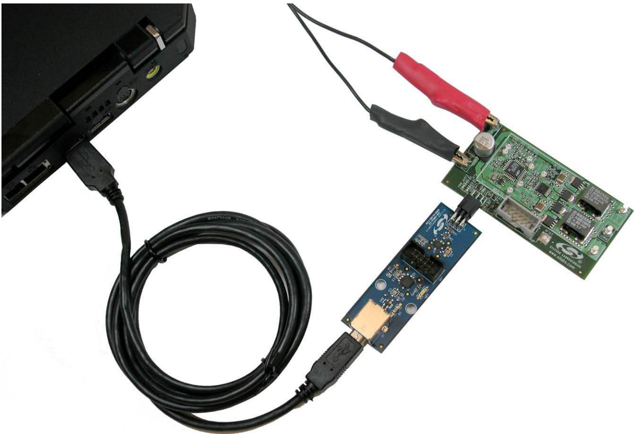
Figure 4. USB to SMBus Bridge Board Connection (Load not Connected)
