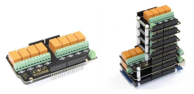
**CANADUINO®** Stackable Relay Shield for Arduino is available as DIY soldering kit with all SMD parts already assembled and trough-hole parts included for DIY assembling.
