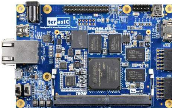
TSOM installed on the TSOM-BB board.
