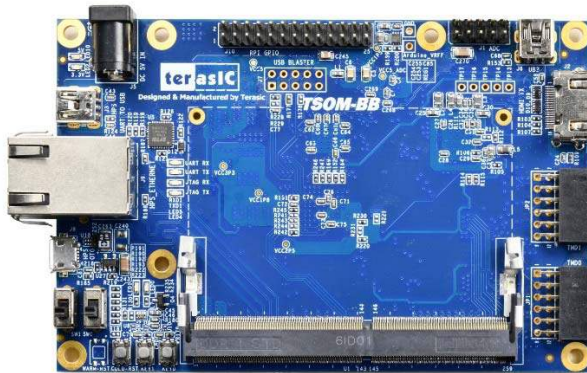
TSOM installed on the TSOM-BB board.
