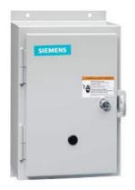
Non-reversing contactor, Size 1 3/4, Three phase full voltage, Contactor amp rating 40A, 3 wire (NO aux included), 110V 50Hz / 120V 60Hz coil, Non-combination type, Enclosure NEMA type 12, Dust/drip proof for indoors, Extra-wide enclosure
