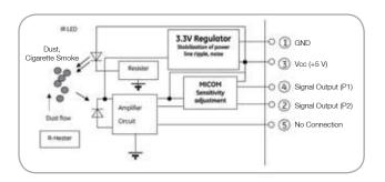
P1: small particle (1~ 2µm), P2: large particle (3~10µm)
