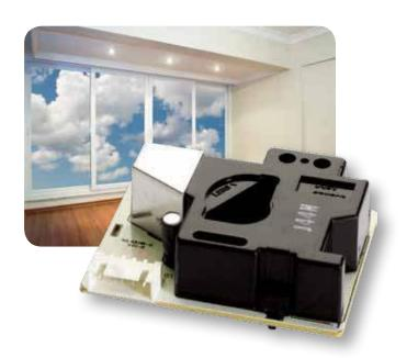
SM-PWM-01A is a dust sensor that detects the dust particle concentration in air by using optical sensing method. An infrared light emitting diode (IR LED) and a photo-sensor are optically arranged in the device. The photo-sensor detects the reflected IR LED light by dust particles in air.
