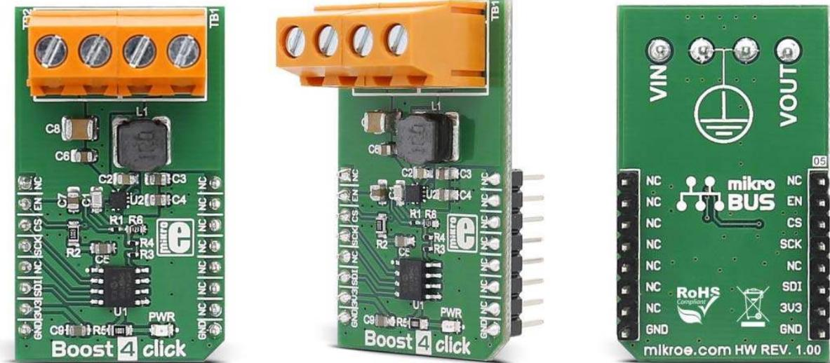
**Boost 4 click** carries the TPS61230A, a high efficiency fully integrated synchronous boost converter from Texas Instruments. The click is designed to run on a 3.3V power supply. Boost 4 click drives the target chip through the digi pot, which has SPI communication with the microcontroller on the system.
