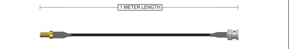
Connector A 132116 SMA Jack Straight Brass Gold + Heatshrink 50 Ohm RG-58 Continuity/Hi-Pot Connector B 031-320 BNC Plug Straight Brass Nickel + Heatshrink
