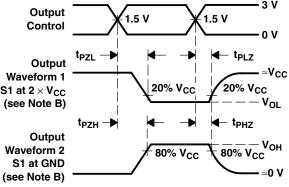
**VOLTAGE WAVEFORMS OUTPUT ENABLE AND DISABLE TIMES**
