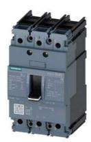
circuit breaker 3VA5 UL frame 125 breaking capacity class S 25kA @ 480 V 3-pole, line protection TM210, FTFM, In=125A overload protection Ir=125A fixed short-circuit protection li=10 x In nut keeper kit on both sides
