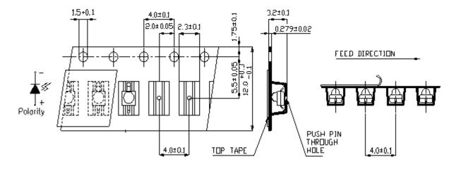
Note: The tolerances unless mentioned are  $\pm 0.1$ , unit=mm.
