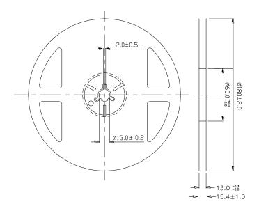
Note: The tolerances unless mentioned are ±0.1, unit=mm
