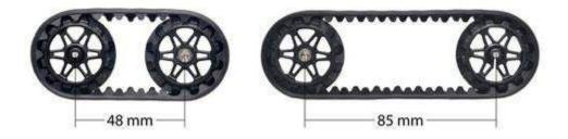
These track sets are similar to the original 22T and 30T track sets, except they replace the old sprockets with newer, spoked versions. This spoked design removes material from several areas near the central hub of the sprocket, which has the advantage of allowing the drive sprocket to be more easily removed from the D-shaft of the motor while still remaining firmly fixed after being press-fit into place.
