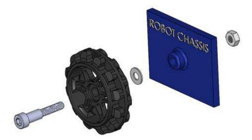
Included are two pairs of shoulder bolts, one with a 5mm threaded portion and one a 12mm threaded portion, so you can pick the pair that is appropriate for your application. You will only use two of the four included shoulder bolts.
