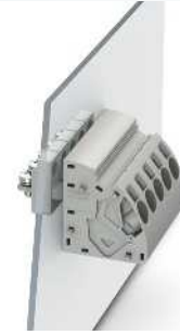
16 mm 2 molded feed-through terminal block, external part with push-in connection, internal part with cable lug connection
