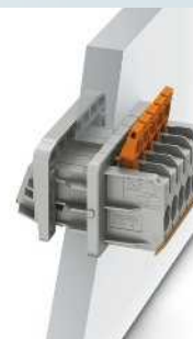
16/6 mm 2 feed-through terminal block, external part with push-lock connection, internal part with push-in connection
