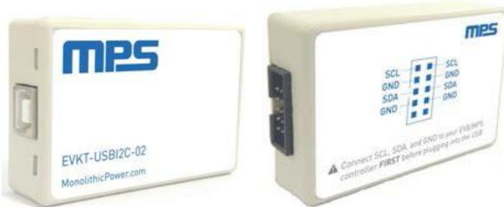
Figure 3: EVKT-USBI2C-02 Communication Interface
