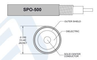
SPO-500 Coax Using Times Microwave Parts PE3C6372-48
