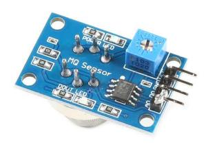
This is the MQ-2 Gas and Smoke Analog Sensor Breakout Board. It's most common use is domestic gas leakage alarms and detectors with a high sensitivity to propane and smoke. The sensing material is  $SNO_2$  (tin oxide) for which the conductivity is lower in clean environments and higher when smoke or flammable gas is present. This is a low-cost sensor for use in a variety of applications.
