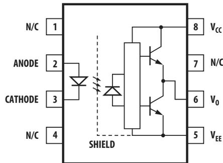
A 0.1  $\mu$ F bypass capacitor must be connected between pins 5 and 8.
