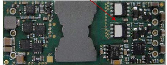
Fig. G: Location of thermocouples for thermal testing
