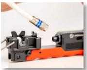
Using specially designed jaws to hold connectors in place while compressing, this **PATENTED** CTF-360XL is designed to hold and compress connectors requiring a full 360 degree support. Perfect tool for long F connectors for RG59/6 cables and F connectors for RG7/11 cables. This tool also features the following:
