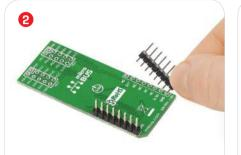
Turn the board upside down so that the bottom side is facing you upwards. Place shorter pins of the header into the appropriate soldering pads.
