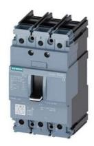
circuit breaker 3VA5 UL frame 125 breaking capacity class H 65kA @ 480 V 3-pole, line protection TM210, FTFM, In=80A overload protection Ir=80A fixed short-circuit protection Ii=10 x In UL489 SB (naval), 50 deg. cel. cable connection on both sides
