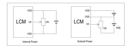
$V_{\text{DD-}}V_0$ : LCD Driving voltage VR:  $10k\sim20k$
