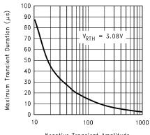
Negative Transient Amplitude,  $V_{RTH} - V_{CC}$  (min) (mV)
