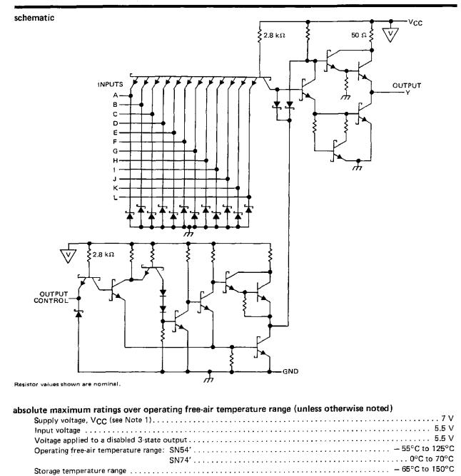
NOTE 1: Voltage values are with respect to network ground terminal.
