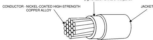
JACKET - RADIATION-CROSSLINKED, MODIFIED ETFE
