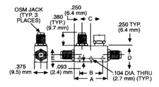
1. All dimensions are ±0.020, except mounting hole diameters (±0.005) and mounting hole location (±0.010).
